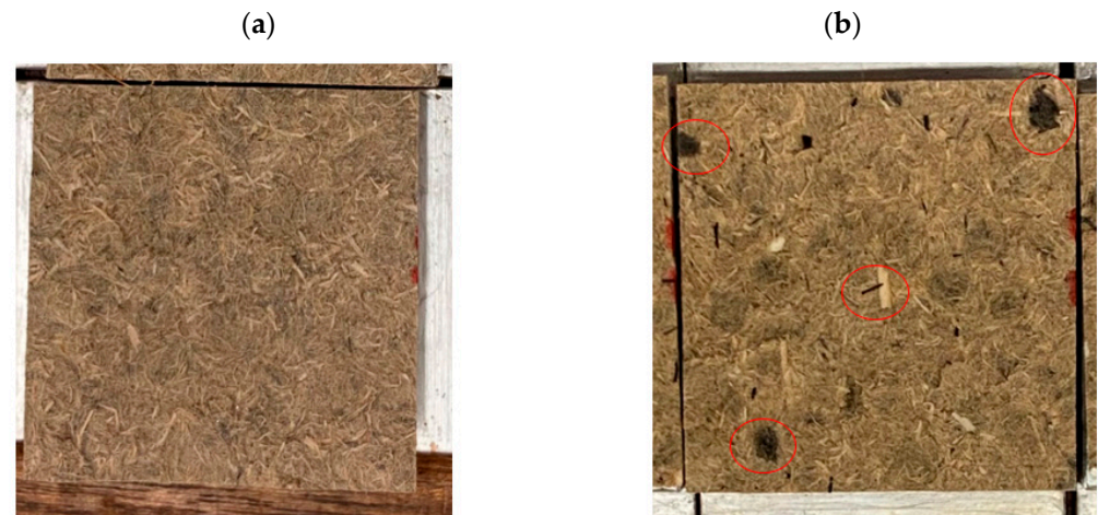
Figure 8. Breaking surface of IB samples after testing. Samples of (a) wet mixed panels and (b) dry mixed panels with red circles highlighting the agglomerates of CF. In both cases, the pictures have been taken from samples containing 5 wt% of CF.
